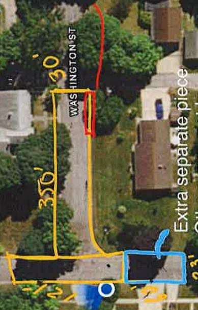
Curbs from Washington up to retaining wall need torn out, they're unlevel and messed up.
